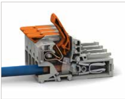
Lift lever to open spring and insert the conductor.
